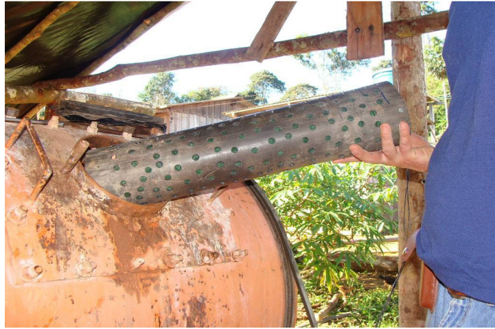
Figure 7 – PVC capsule containing the nylon screen with the activated carbon
