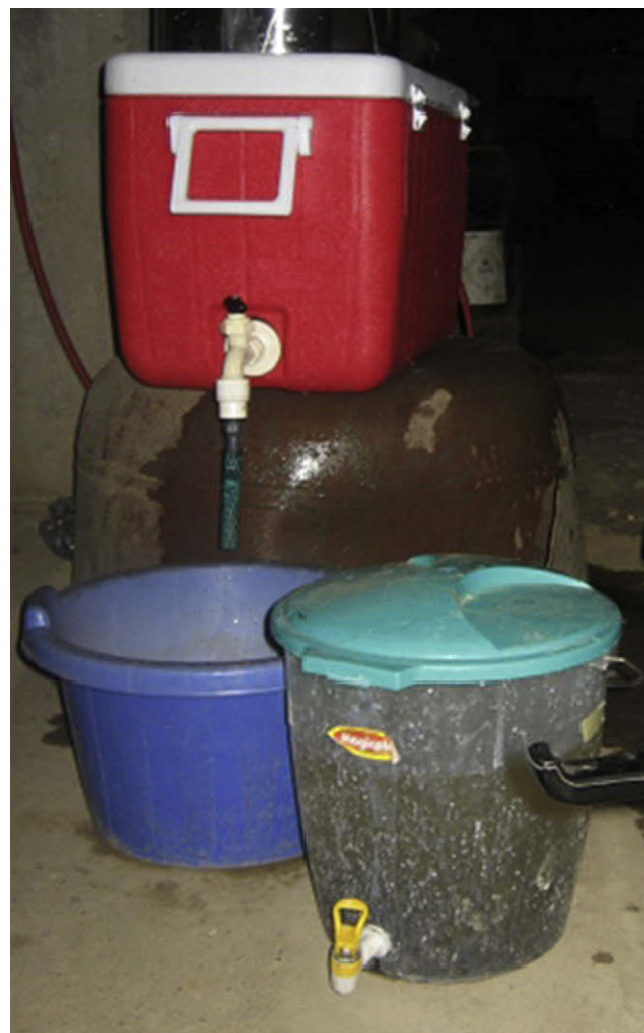
Fig. 5. Thermo-box used to strip gold from activated carbon.
